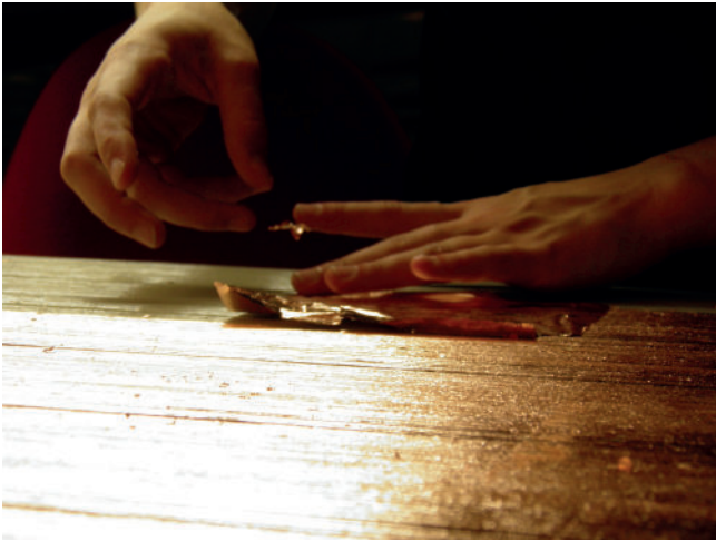
Copper leaf deposition on larch wood - SUAGE collection - SIGébène
